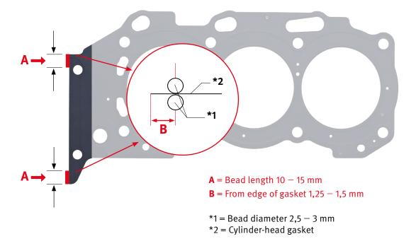
Gasket location on right cylinder bank shown. Application on left cylinder bank similar.
