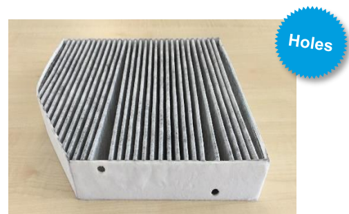
Image 2: The OE filters have two holes. Two pins placed in the housing can ingress in the filter.
